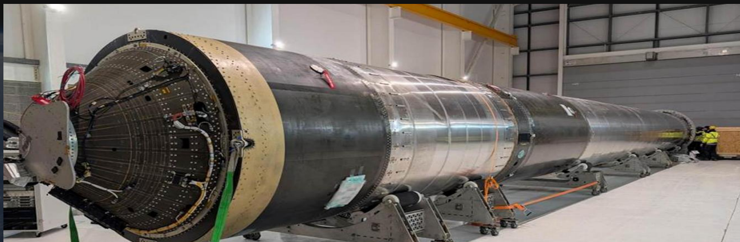
RFA ONE launch vehicle in the SaxaVord integration hall – S1/S2 integrated, April 2026
