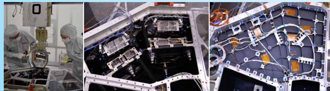
Instrument Optical Unit structure integrated with the pre-assembled Mirrors and Prisms, forming the EnMAP Spectrometer
