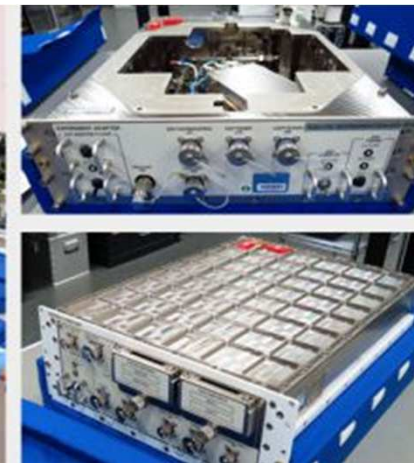
Components of the “PK-4” plasma crystal laboratory: experiment unit, rack drawers for electricity supplies, communications and data collection
