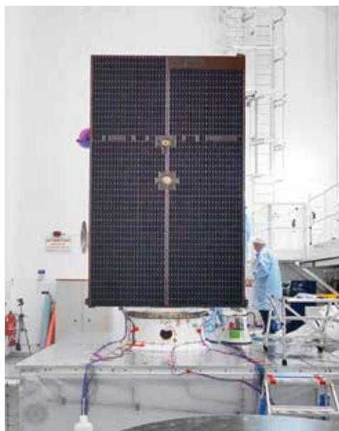
The Environmental Mapping and Analysis Program (EnMAP) describes the Earth's environment on a global scale. The hyperspectral imager (HSI) measures solar radiation reflected from the earth's surface as a high-resolution continuous spectrum from visible light to short-wave infrared light.
