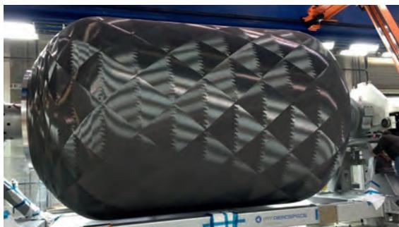
The CFRP booster demonstrator during the winding process at DLR-ZIP (left) and after burst testing in the testing pit at the Materials Testing Institute (MPA) in Stuttgart (above).
