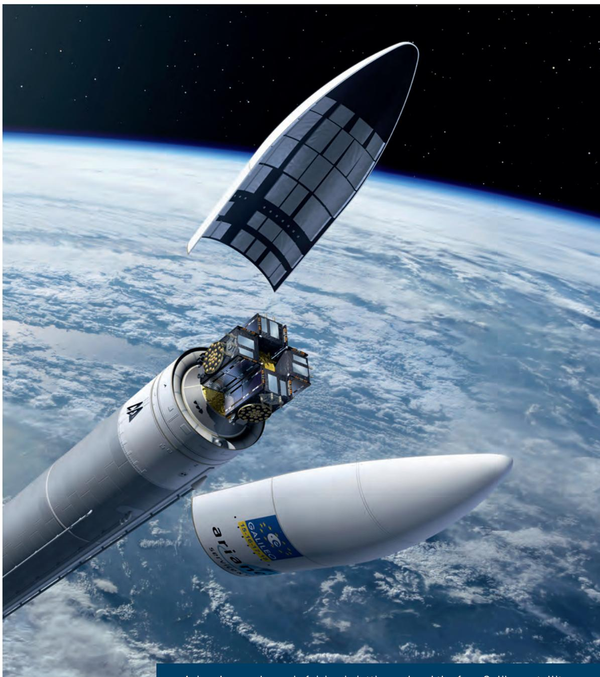
Ariane's aerodynamic fairing is jettisoned and the four Galileo satellites 'see' space for the first time
