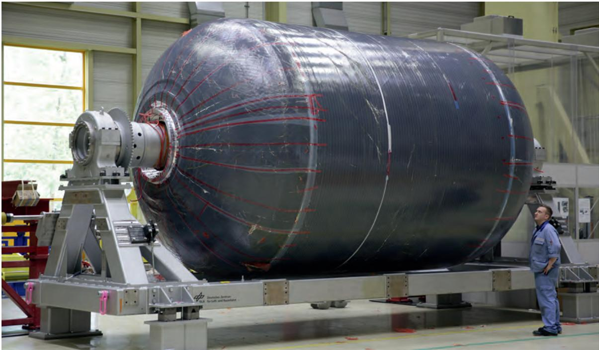
Booster made from carbon fibre-reinforced plastic (CRP) in a partnership between DLR and MT Aerospace
