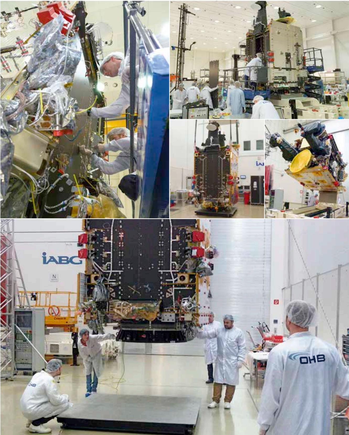
Hispasat AG1 at the end of the integration phase at OHB System AG's clean room in Bremen (top) and at the beginning of environmental impact testing at the IABG space center in Ottobrunn (bottom pictures).
