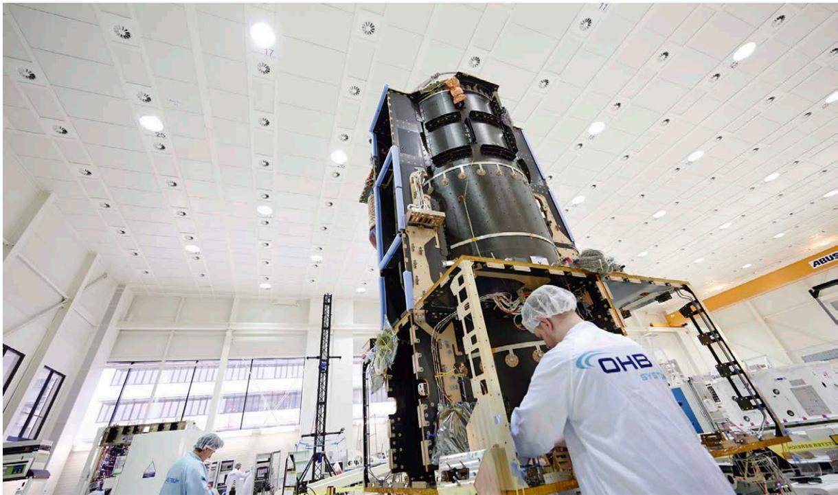
ExoMars TGO Core core module in the cleanroom at OHB
