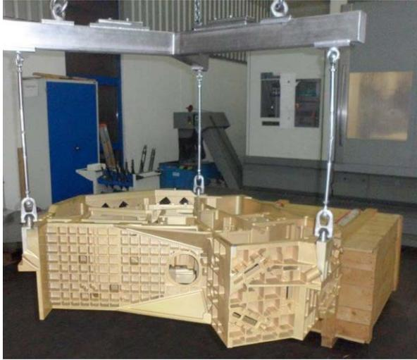
The central highly complex structural part for holding the optical components of the hyper-spectral instrument on EnMAP
