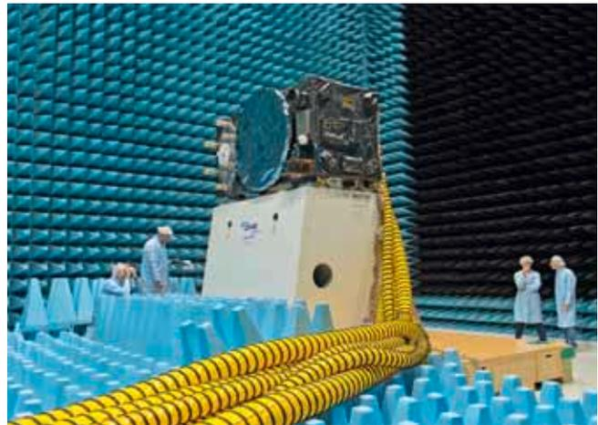
Galileo FOC FM1 during preparations for the PIM test
