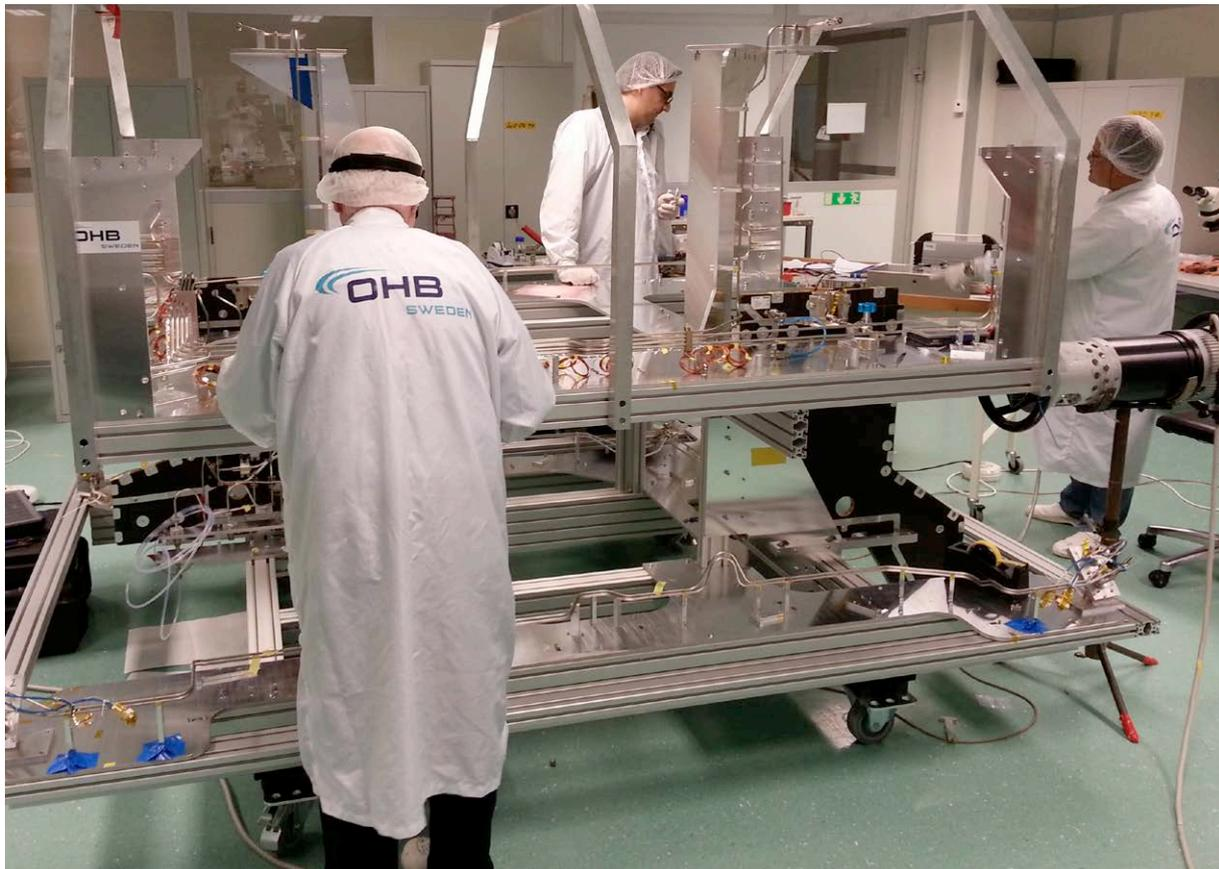
Fixing and testing of the position control system for the SmallGEO satellite at OHB Sweden
