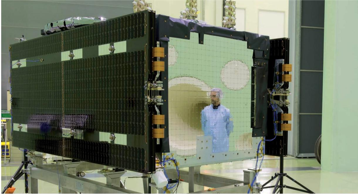
Second Galileo\* Full Operational Capability (FOC) satellite being prepared for acoustic testing, simulating the noise of a rocket launch, inside the Large European Acoustic Facility, LEAF, of the ESTEC Test Centre in early September 2013.
