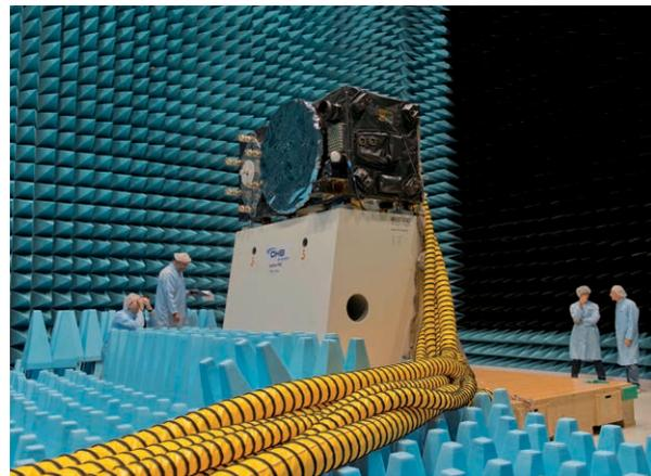
Galileo\* Full Operational Capability (FOC) satellite first flight model, FM1, being prepared for ‘passive intermodulation testing’ within the Maxwell electromagnetic test facility inside the ESTEC Test Centre at the end of August 2013.
