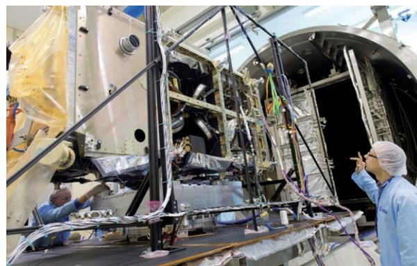
The first Galileo\* Full Operational Capability (FOC) satellite beside the Phenix test chamber in the ESTEC Test Centre in October 2013, being readied for its five-week-long thermal vacuum test. Note the thermal tent visible inside the chamber, used to reproduce the temperature extremes of Earth orbit.
