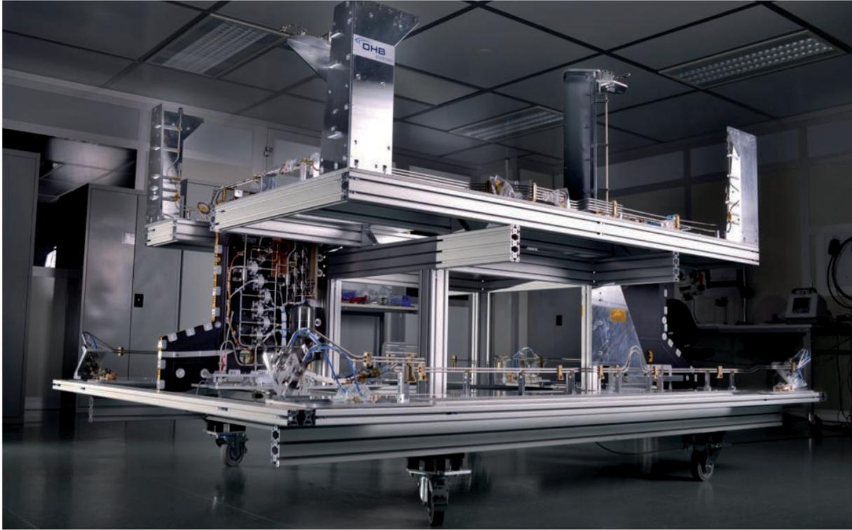
The SmallGEO Electric Propulsion Tubing System just before delivery to Bremen.
