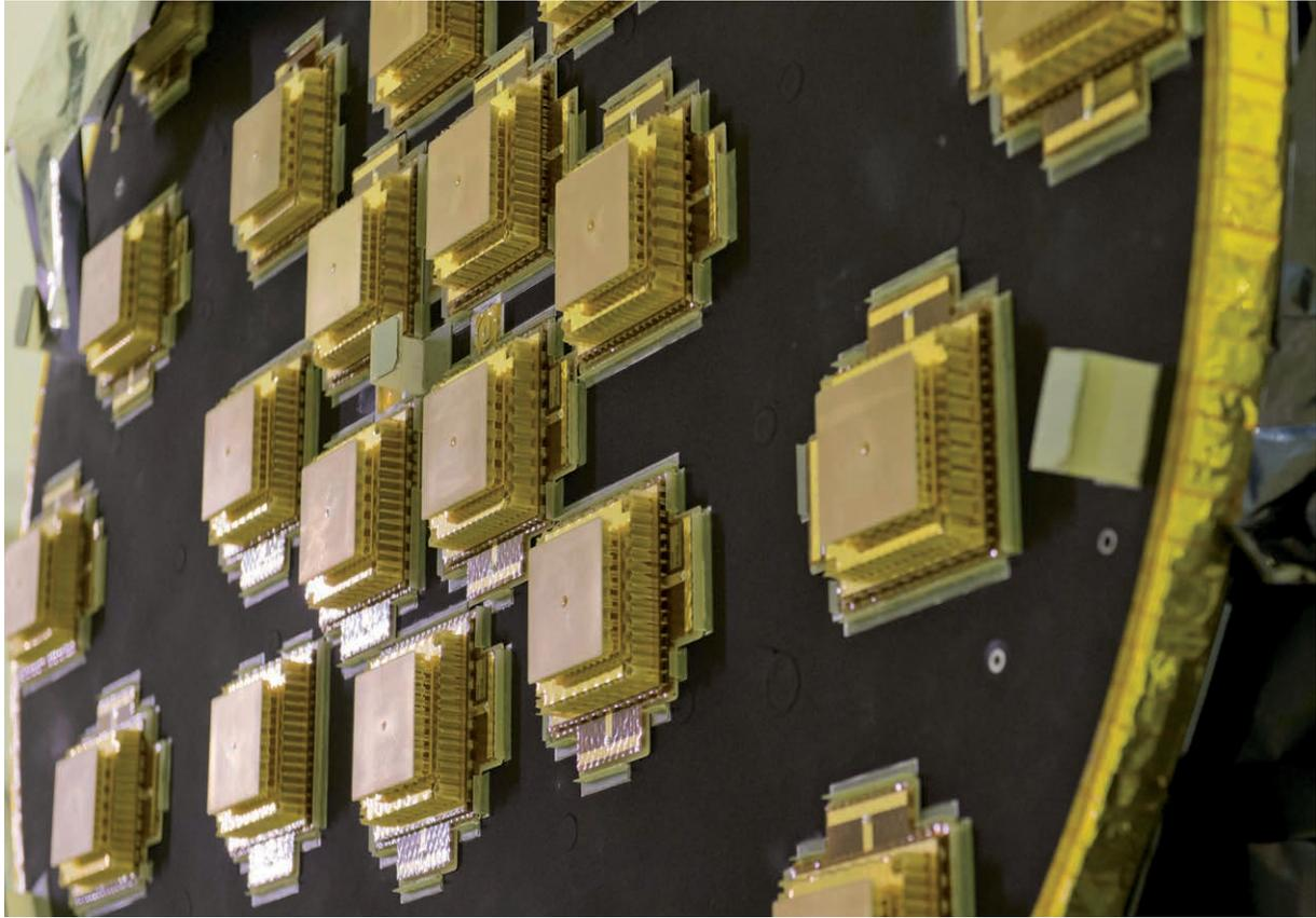
Galileo\* Full Operational Capability Flight Model 2, FM2, satellite's main L-band antenna used for broadcasting navigation messages, seen during preparation for a mass property test at the ESTEC Test Centre at the end of August 2013.
