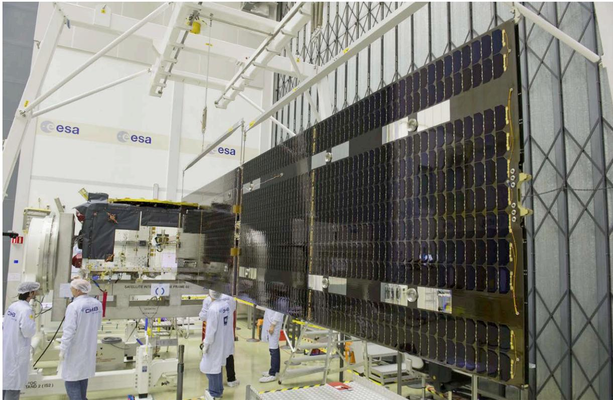
Function testing of the first Galileo\* FOC satellite "Doresa" at ESA's ETS.
