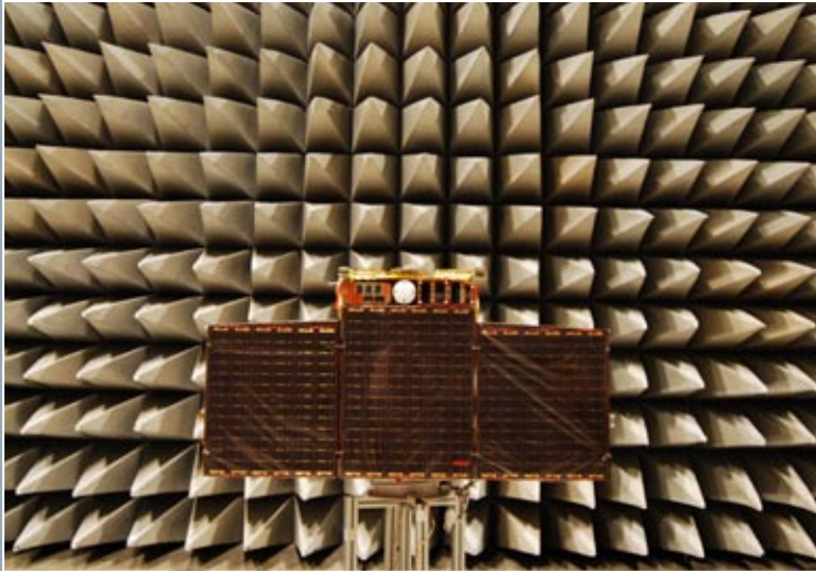
TET-1 (shown here during EMC trial) sends technological models into space for testing
