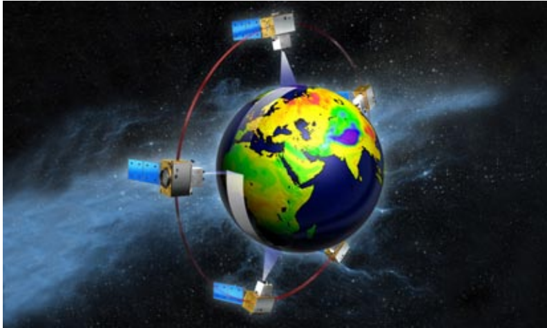
CarbonSat constellation: system for satellite-based monitoring of CO 2 and methane
