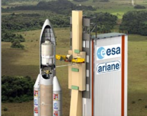
Ariane-5 launch vehicle with elongated fairing to protect the ATV bound for space.
