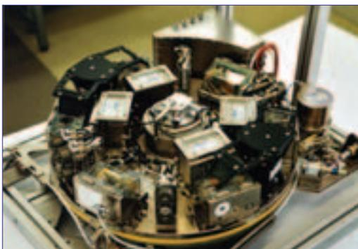
Centrifuge for the ESA BIOLAB research facility on board to ISS
