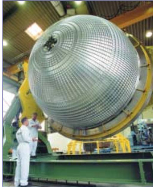
*Component for the liquid hydrogen tank of the upper stage of the Ariane 5*
