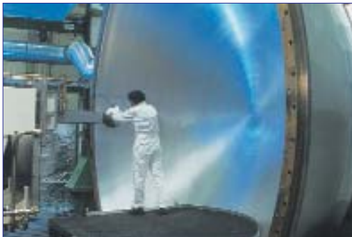
Spin-forming the cryo tank dome of the Ariane 5
