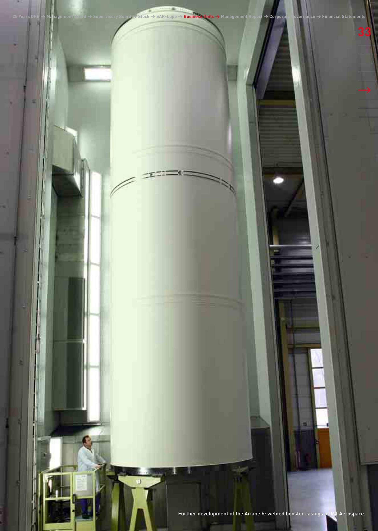
Further development of the Ariane 5: welded booster casings at MT Aerospace.
