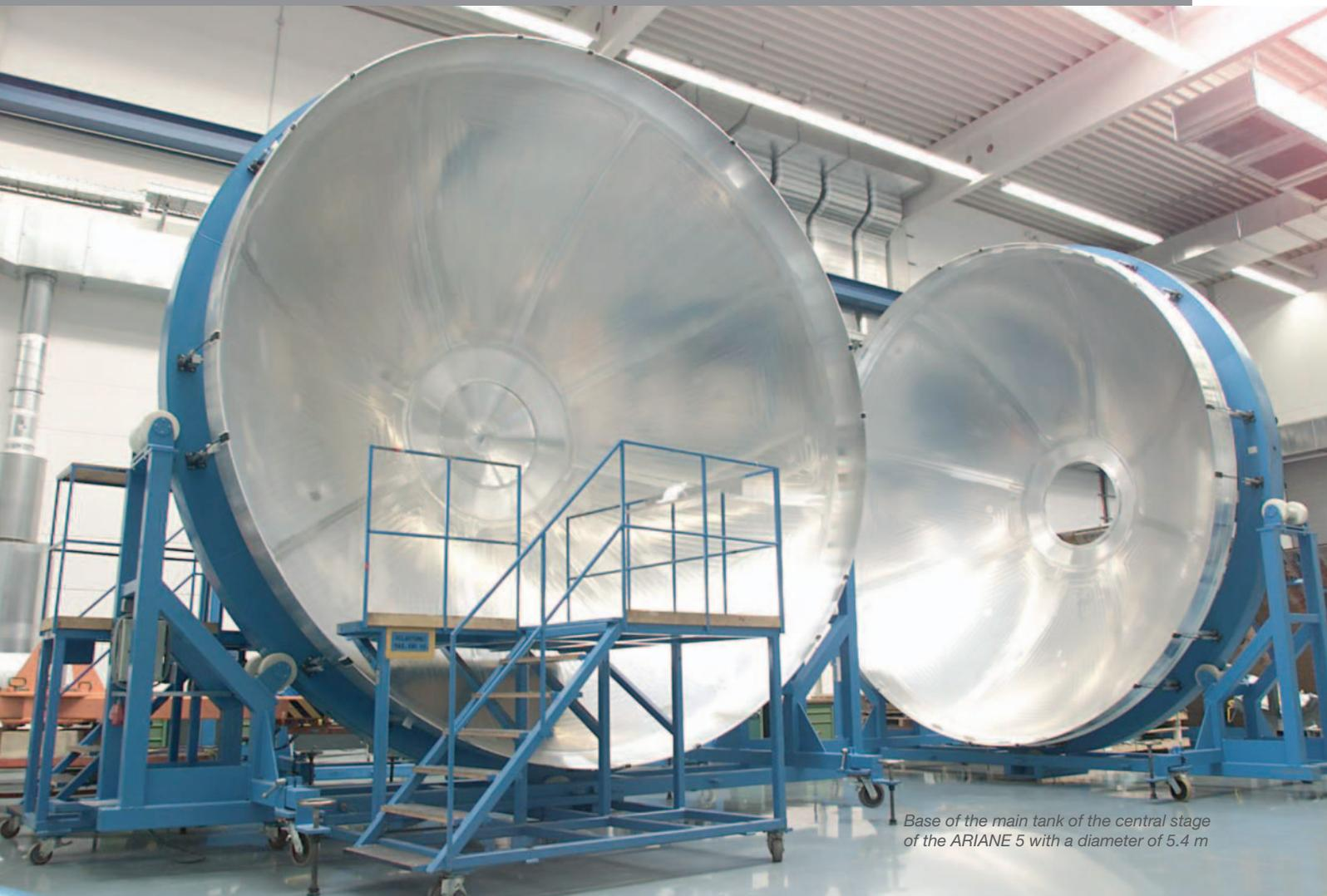
*Base of the main tank of the central stage of the ARIANE 5 with a diameter of 5.4 m*
