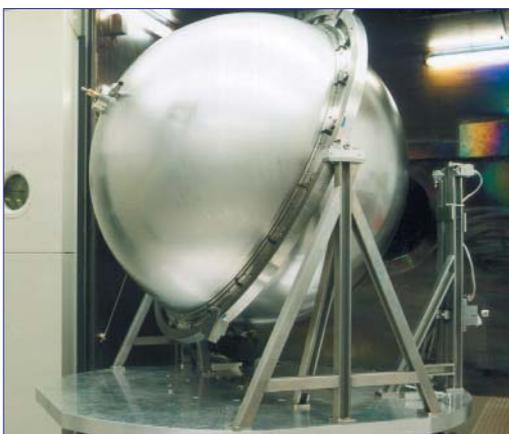
Fuel tank for the Automated Transfer Vehicle (ATV)
