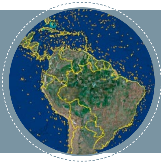
Tracking global shipping by means of satellite-based AIS data
