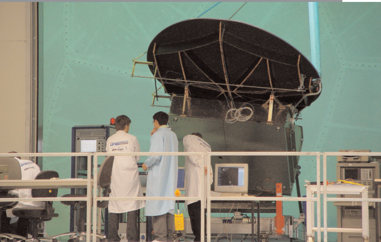
SAR-Lupe Engineering Model during SAR End-to-End Test.
