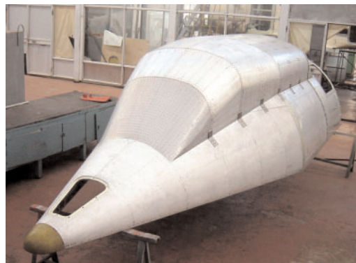
COSMOS fairing: Modifications were necessary for the payload fairing of the COSMOS launchers, which are to be used for putting the SAR-Lupe satellites into orbit. A reference flight with the revised fairing is scheduled for early 2005.
