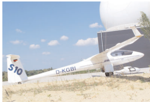
The Stemme S 10 motor glider is an experimentation vehicle for the development of manned/unmanned drones (CONDOR).
