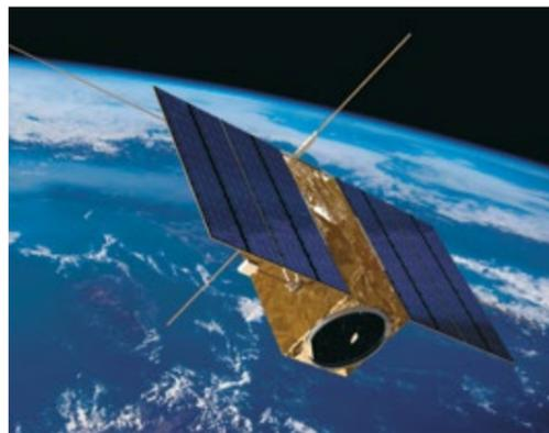
EAGLET 1 is the in-orbit validation of a nanosat developed in accordance with an industrial approach for reliability and performance. The launch marked an important milestone in the deployment of the EAGLET constellation. The total mass is less than 5 kilograms. The satellite has a precise attitude control system based on Earth, Sun and star tracking and GPS sensors.
