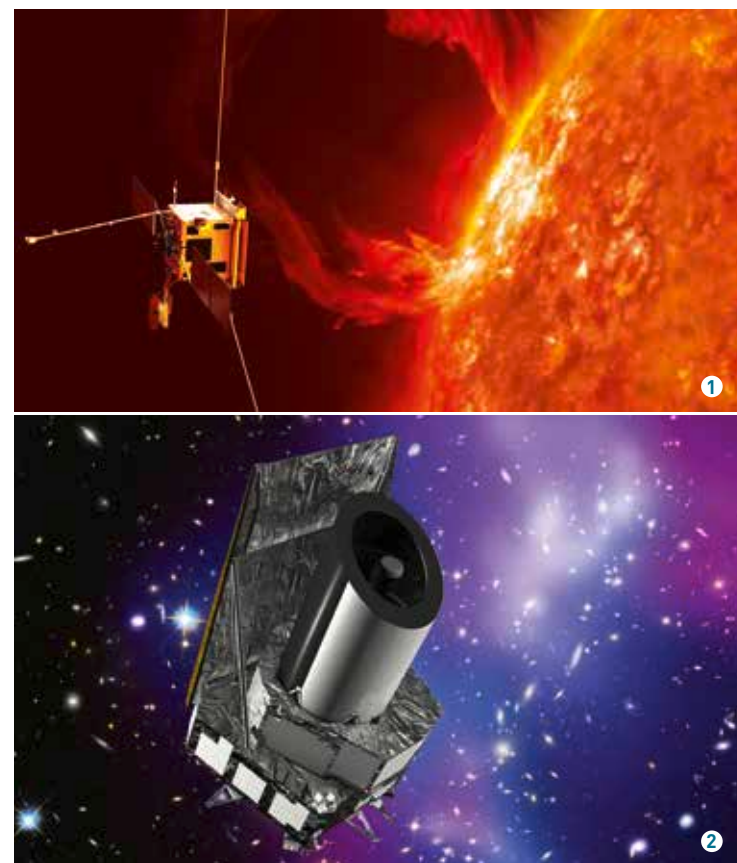
The Solar Orbiter will approach the sun to a distance of 45 million kilometres, thus coming closer than all other space vehicles previously sent out by mankind, even closer than Mercury, the planet nearest to the sun (1). Euclid aims to unravel the mysteries of dark energy and dark matter (2). PLATO will involve the use of 34 independent small telescopes and cameras (3).
