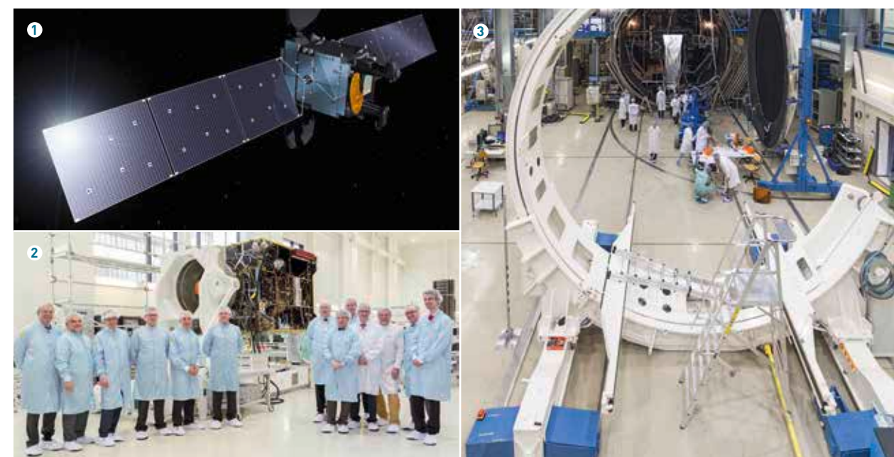
Première: in the form of the H36W-1, the first geostationary satellite based on the SmallGEO platform is now in operation(1). SmallGEO team in the clean room at OHB in Bremen (2). The innovative electric and cold gas propulsion systems come from OHB Sweden. LuxSpace is on board with its telecommand, telemetry & ranging system while OHB Italia supplied the control unit for the Tesat Spacecom payload, for example (3).
