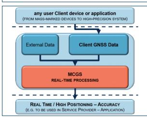
The performance of GNSS products and services strongly depends on the used GNSS receiver quality and the used positioning technique. Stand-alone mass-market receivers usually perform single point positioning based on code pseudoranges on a single frequency enabling a typical positioning accuracy of some metres. The major error contributions caused by un-modelled satellite errors, signal propagation effects as well as the receiver performance.
