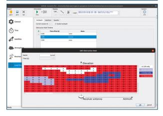
GIPSIE is a highly flexible and powerful GNSS simulation environment that provides the possibility to generate simulated GNSS constellations and IF signals for various user-defined scenarios including complex trajectories and environments. All settings can be made within the userfriendly and intuitive graphical user interface or within an easy-to-read configuration file.
